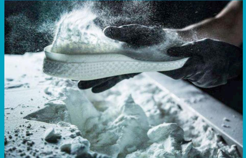
*Figure 5: Shoe silhouette created using SLS. [5]*
